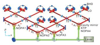
**Figure 2** (Color online) Schematic of experimental setup for CV eight-partite cluster state generation. T: transmission efficient of beam splitter, Boxes including i are Fourier transforms (90° rotations in phase space), -i is a  $-90^{\circ}$  rotation, and -1 is a  $180^{\circ}$  rotation, BHD: balanced homodyne detector.
